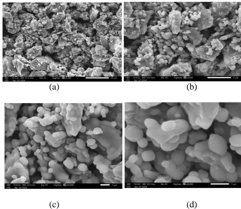
**Figure 3.** SEM images of iron sand and barium hexaferrite (4:1) at magnifications (a) 2,500x, (b) 5,000x, (c) 10,000x, and (d) 20,000x.
