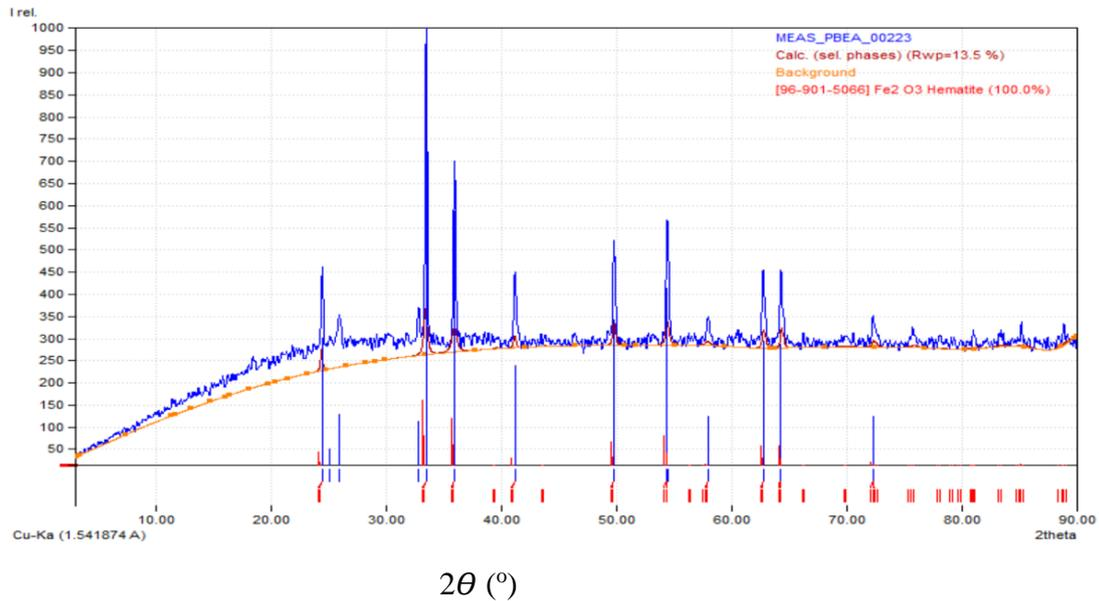
**Figure 2.** Matching XRD results with Match!4 results on iron sand and barium hexaferrite materials with a sample composition of (4:1).
