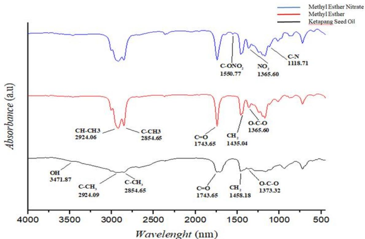
Figure 4. FTIR spectrum
