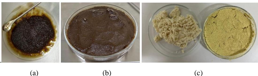
Figure 1. Prior to the bleaching procedure, (a) rice straw hemicellulose, (b) rice husk hemicellulose, and (c) rice straw and husk hemicellulose following the bleaching process.
