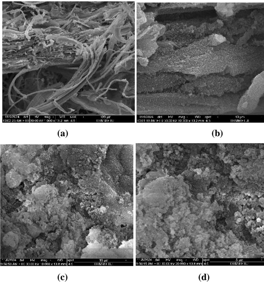
Figure 3. SEM Results (a) Rice Straw Hemicellulose Magnification 100 $\mu$  and (b) Magnification 10 $\mu$ , (c) Rice Husk Hemicellulose Magnification 10 $\mu$  (d) Rice Husk Hemicellulose Magnification 5 $\mu$
