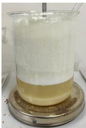
Figure 2. Bleaching Process using H<sub>2</sub>O<sub>2</sub>
