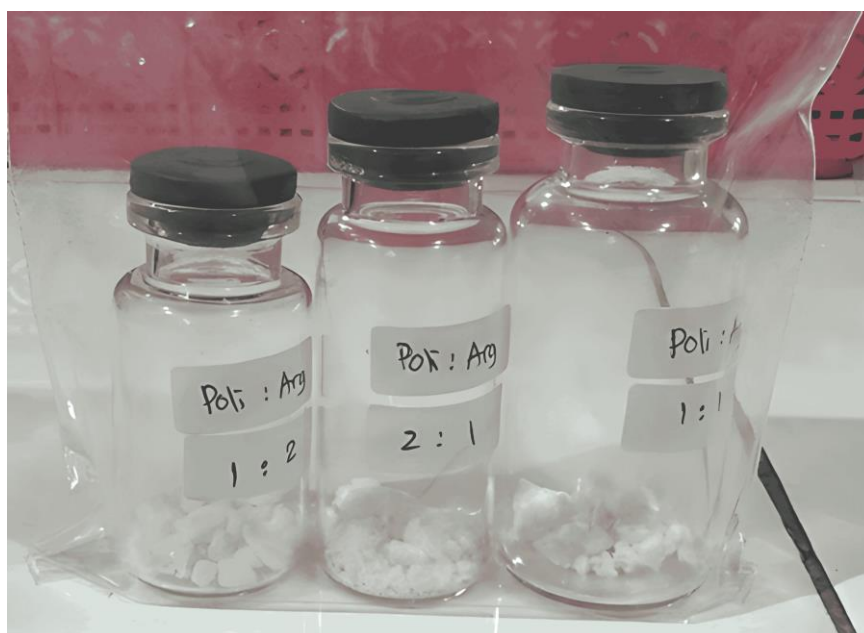
Figure 4. Photographic images of poly(GM-co-EGD) polymers after lipase immobilization at different polymer-to-enzyme ratios: (a) 1:1, (b) 1:2, (c) 2:1.
