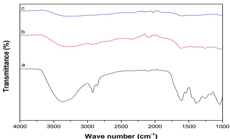
**Figure 4.** FTIR spectra of (a) MLE, (b) Corrosion product in 1 M HCl + mild steel + MLE 6 g/L, and (c) Corrosion product in 1 M HCl + mild steel + MLE 6 g/L + potassium iodide 0.4 g/L
