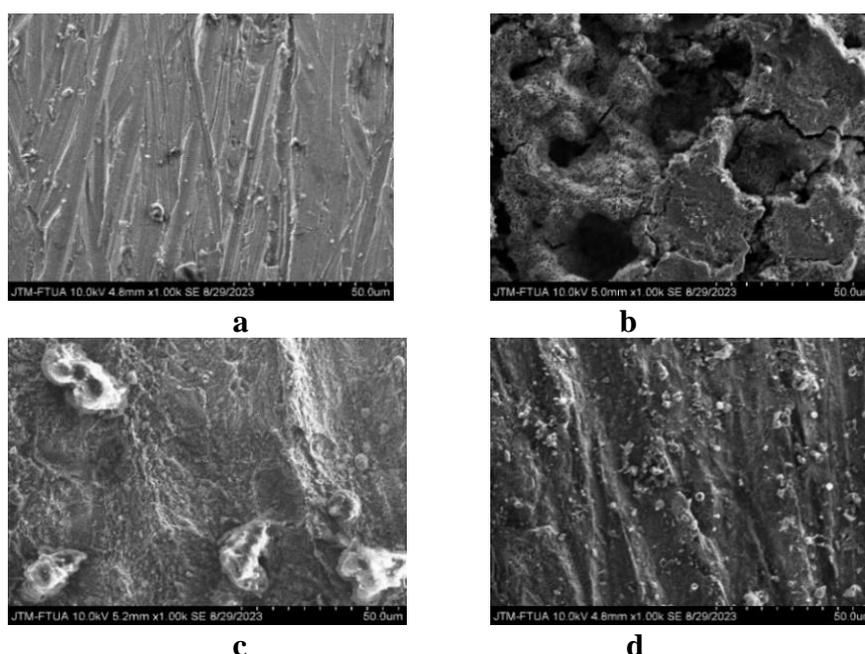
**Figure 5.** Surface morphology of mild steel at a magnification of 1.000x after 6 days: (a) before immersion, (b) immersion in HCl without inhibitor, (c) immersion in MLE, and (d) immersion in MLE and iodide
