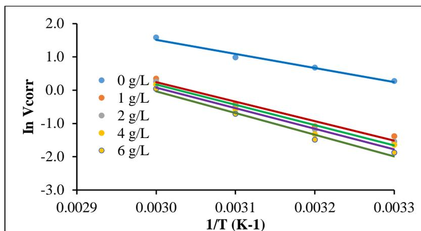
**Figure 3.** Arrhenius plots for the corrosion of mild steel in a 1 M HCl solution without and with the addition of MLE and potassium iodide at various concentrations
