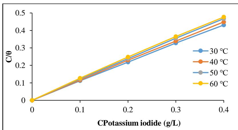
**Figure 2.** The Langmuir adsorption isotherm graph for the corrosion of mild steel with MLE and potassium iodide in a 1 M HCl solution
