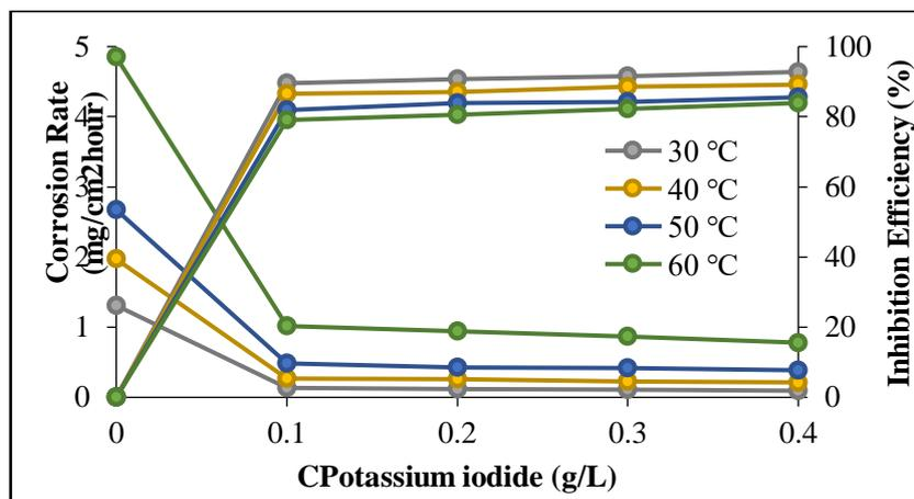
**Figure 1.** The Influence of Various Concentrations of Potassium Iodide on the Corrosion Rate ( $V_{\text{corr}}$ ) and Inhibition Efficiency (%IE) in 1 M HCl
