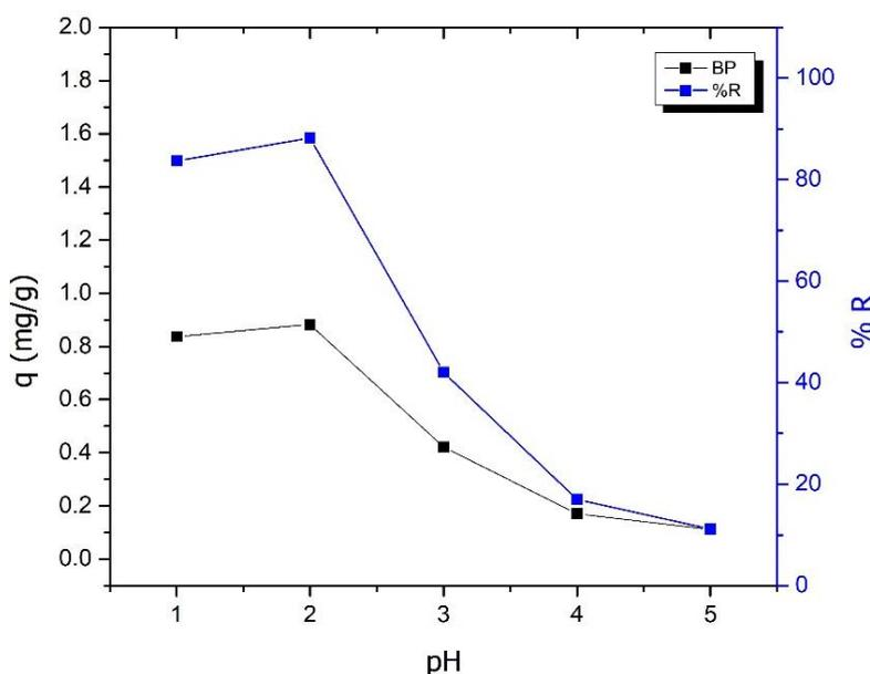
Figure 3. Effect of pH on the adsorption capacity of IC dye ( $C_0$ :  $10 \text{ mg L}^{-1}$  ; biosorbent mass: 0,1 gram; contact time: 60 minutes ; adsorption temperature:  $25 \text{ }^\circ\text{C}$  ; volume: 10 mL; particle size:  $36 \text{ }\mu\text{m}$  ; and 100 rpm)
