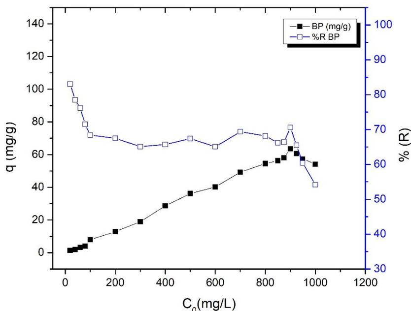
Figure 5. Effect of IC dye initial concentration on adsorption capacity (pH: 2 ; biosorbent mass: 0.1 gram ; contact time: 60 minutes ; adsorption temperature: 25 °C ; volume: 10 mL ; particle size: 36 μm ; and 100 rpm)
