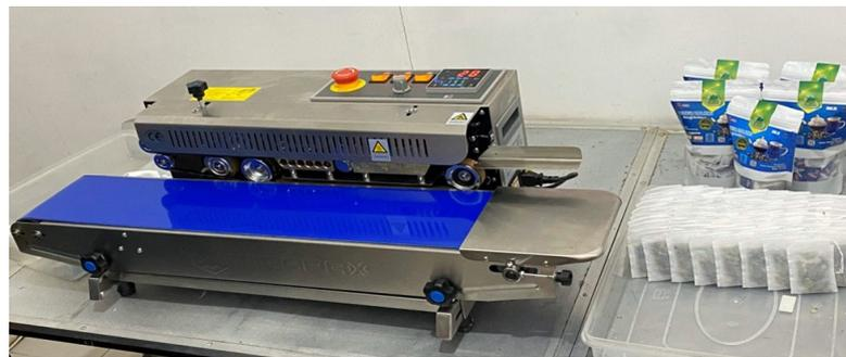
**Gambar 5. Introduksi Continuous Band Sealer**
