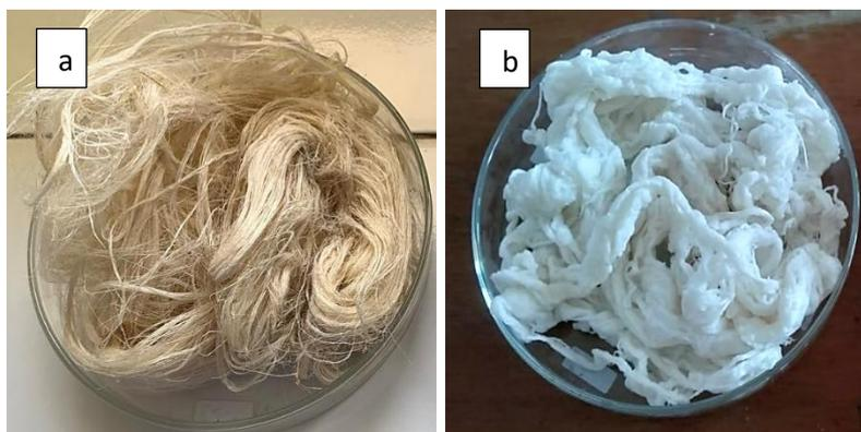
**Figure 1.** The Untreated PALF (a) Treated PALF (b)
