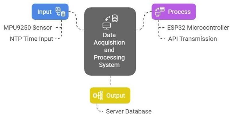
**Figure 1.** Block diagram of instrument
