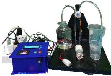
**Fig 7.** Arduino-based Flowmeter Sensor Trainer for Measuring Water Flow
