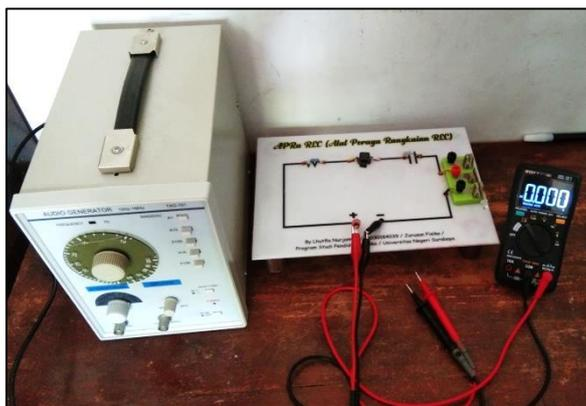
**Figure 6.** RLC circuit props
