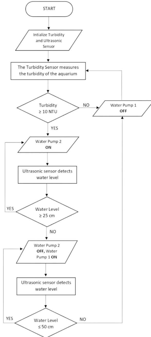
**Figure 3.** Turbidity sensor software design.
