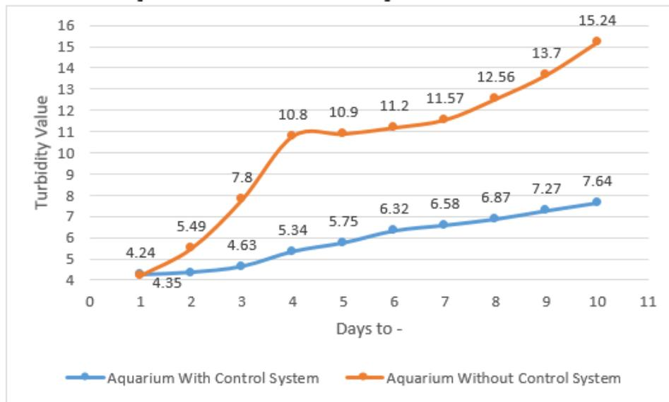
**Figure 7.** A comparison graph of measurement values for aquarium water turbidity over 10 days
