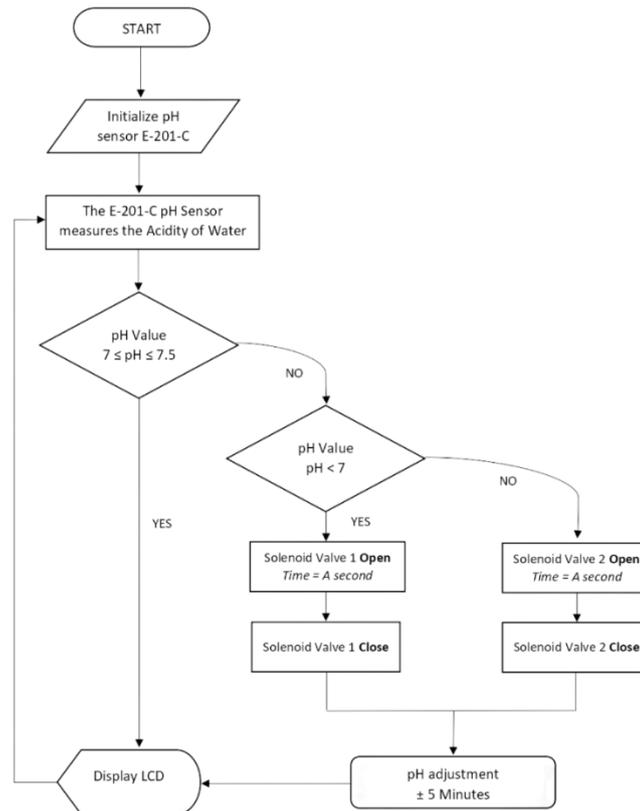
**Figure 4.** pH sensor software design.
