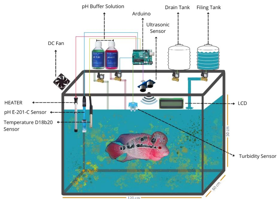
**Figure 1.** Overall hardware system design.
