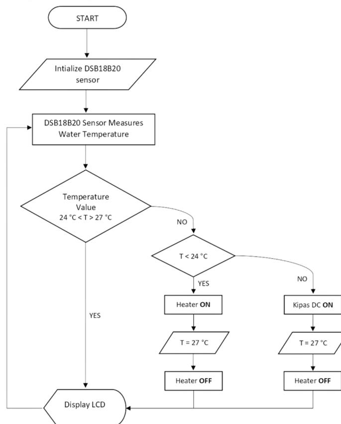
**Figure 2.** Temperature sensor software design.
