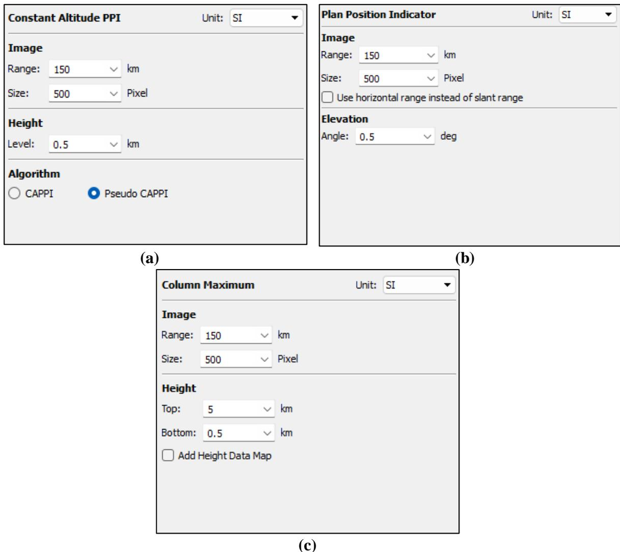
**Figure 2.** Setting of the radar product used (a) CAPPI, (b) PPI, (c) CMAX
