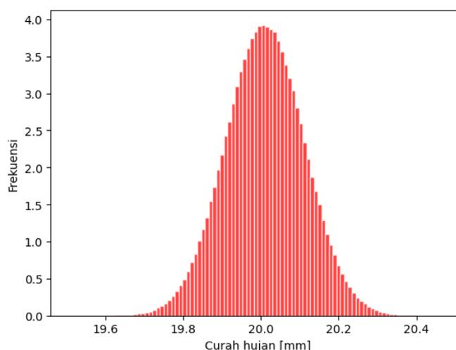
**Figure 3a.** Case 1 - The histogram represents the PDF generated for rainfall measurement using Monte Carlo simulation (using a calibrated dial caliper).
