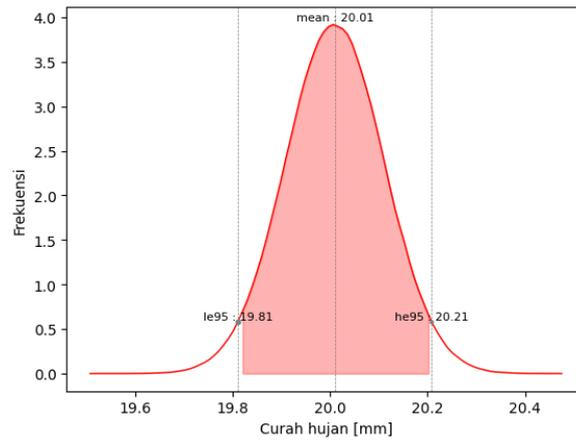
**Figure 3b.** Case 1 - The low endpoint and high endpoint graphs for a coverage factor of 95% represent the PDF generated for rainfall measurement using Monte Carlo simulation (using a calibrated dial caliper).
