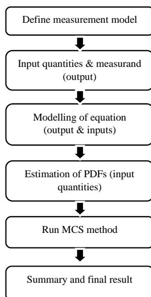
**Figure 2.** Steps to calculate uncertainty of measurement using MCS
