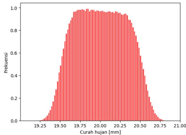
**Figure 4a.** Case 2 - The histogram represents the PDF generated for rainfall measurement using Monte Carlo simulation (using an uncertified ruler).
