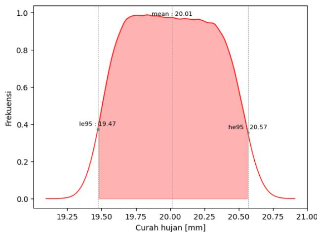
**Figure 4b.** Case 2 - The low endpoint and high endpoint graphs for a coverage factor of 95% represent the PDF generated for rain gauge measurement using Monte Carlo simulation (using an uncertified ruler).
