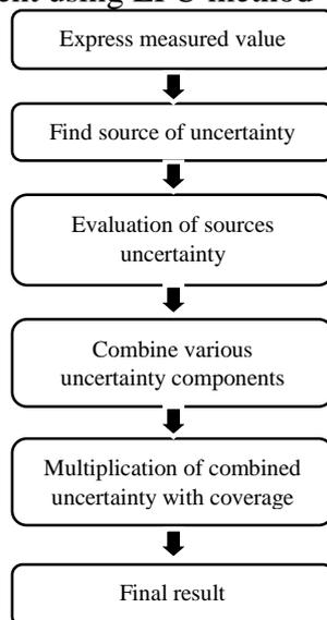
**Figure 1.** Steps to calculate uncertainty of measurement using LPU/ GUM
