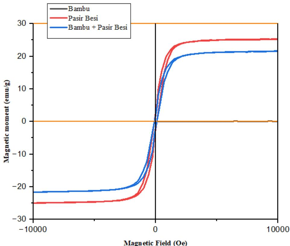
**Figure 2.** Hysteresis Loop of bamboo; natural iron sand; bamboo + natural iron sand
