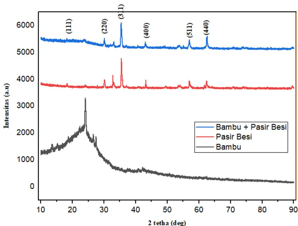
**Figure 1.** Diffraction pattern of bamboo XRD; natural iron sand; bamboo + natural iron sand
