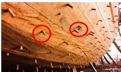
Figure 14. Wooden pegs in the hull
