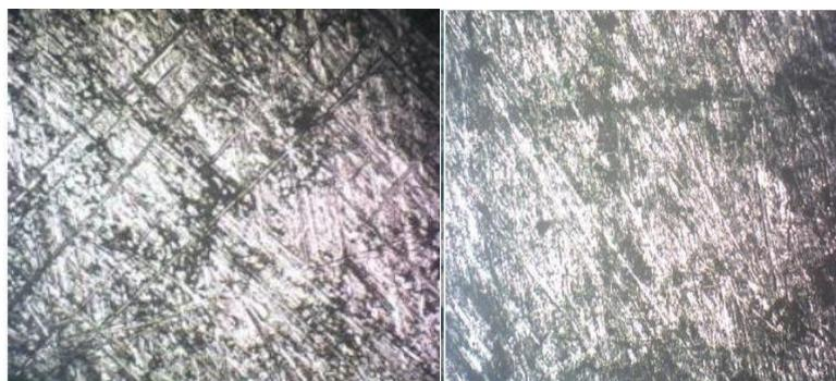
**Figure 7.** Visual Analysis of the Condition of Carbon Steel Metal Coated with Tribofilm Material with 60% wt Activated Carbon Variations Soaked in 3.5% NaCl Ocean Media
