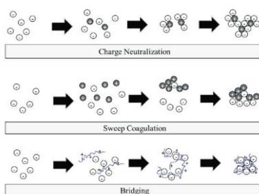
**Figure 2.** Coagulation Process
